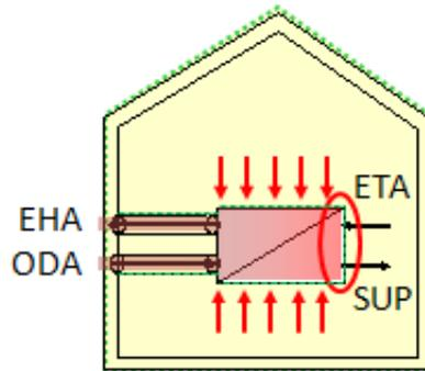
Figure 1(b) Industry calculation of heat recovery rate based on the **supply air side**
