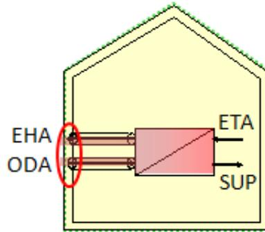
Figure 1(a) PHI calculation of heat recovery rate based on the **exhaust air side**
